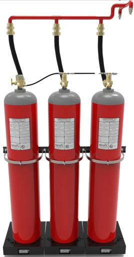
**MORX weighing device** is able to monitor and provide signals of the filled and unfilled cylinder weight. When the cylinder weight is less than a pre determined level, a signal is sent to the control panel and indicating lights turn on.
